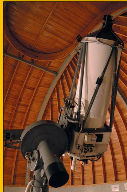
**Figure 1:** The Mayer 65-cm reflecting telescope located at Ondřejov observatory, CCD camera in the primary focus. (Photo Kamil Hornoch)
