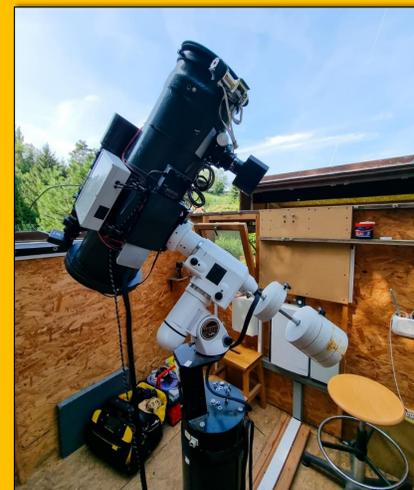
**Figure 5:** The 20-cm Newtonian telescope with CCD camera MII G2-1600 at South-Moravian Observatory. (Photo Reinhold F. Auer)
