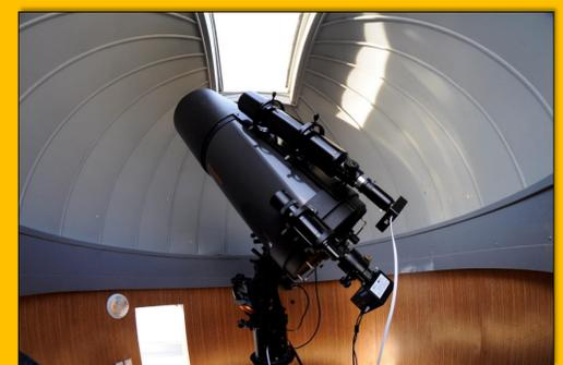
**Figure 3:** The 35-cm SCT Celestron telescope with CCD camera MII G2-1600 at Valašské Meziříčí observatory. (Photo Ladislav Šmelcer)
