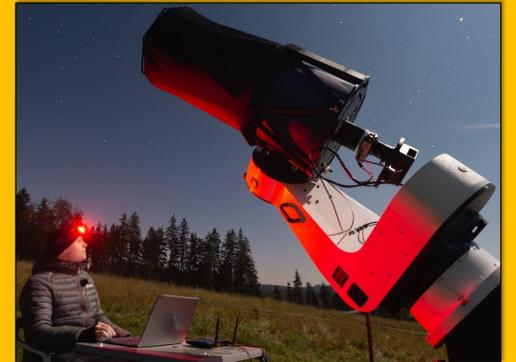
**Figure 2:** The 40-cm Ritchey-Chrétien telescope at Dark Sky observatory in Beskydy, CCD camera MII C3 Pro mono. (Photo Tomáš Hynek)
