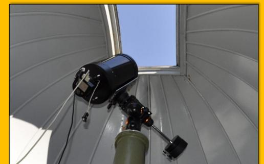
**Figure 4:** The 28-cm Celestron telescope at Valašské Meziříčí observatory with the MII G2-4000 CCD camera. (Photo Ladislav Šmelcer)
